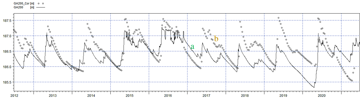
Figure 4: Calibration of the groundwater component (a) Groundwater table simulated by MIKE SHE and (b) Comparison of the modelled and observed hydraulic heads.
