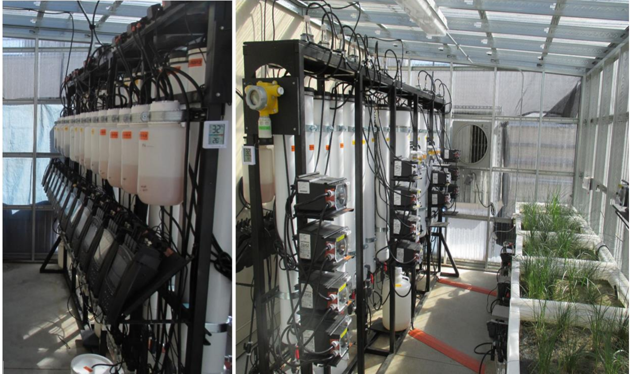
Figure 2. Lab-scale treatability study setup. Left: Sample reservoirs, multi-meters, and flow-through cells on the back side of the rack. Right: Columns are on the front side of the rack and treatment wetlands on the right.
