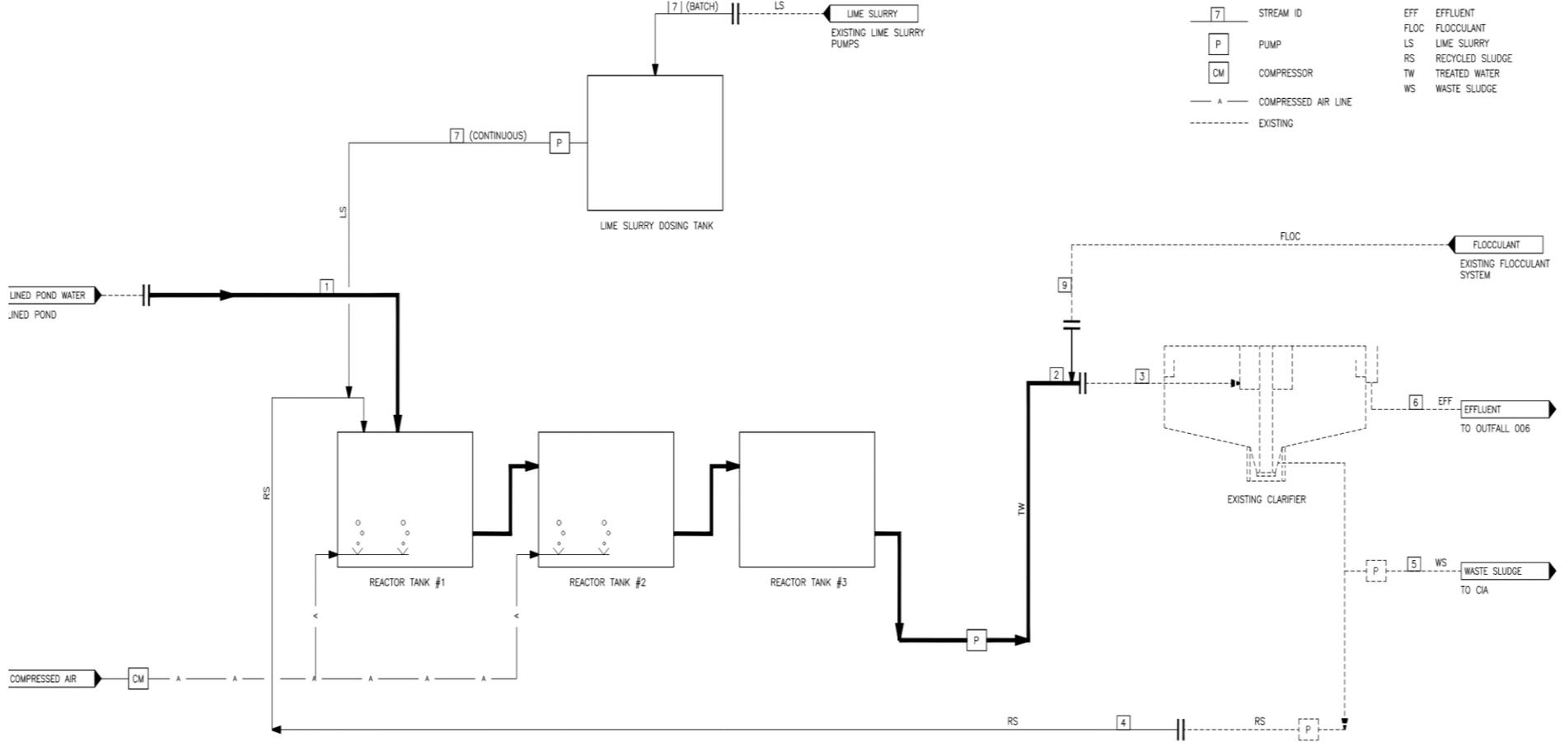
Figure 3: Process Flow Diagram TTS
