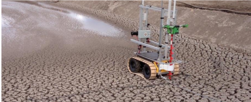
Figure 4: RTC-II UGV drilling on an oil sands tailings deposit
