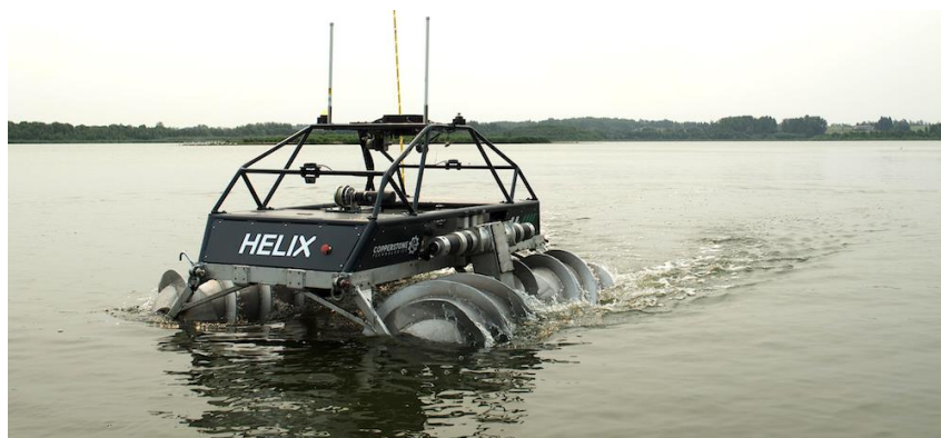
Figure 5: Screw-drive amphibious robot moving across a lake
