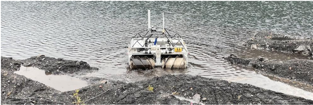
Figure 8: HELIX Neptune deployed in a pit-lake with YSI EXO Sonde
