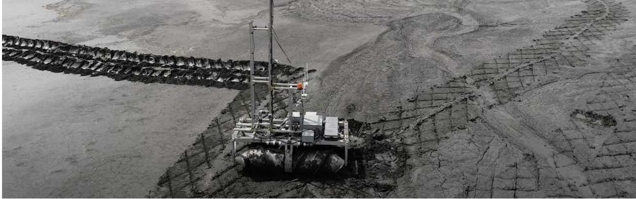
Figure 9: HELIX Neptune deployed in a pit-lake with YSI EXO Sonde
