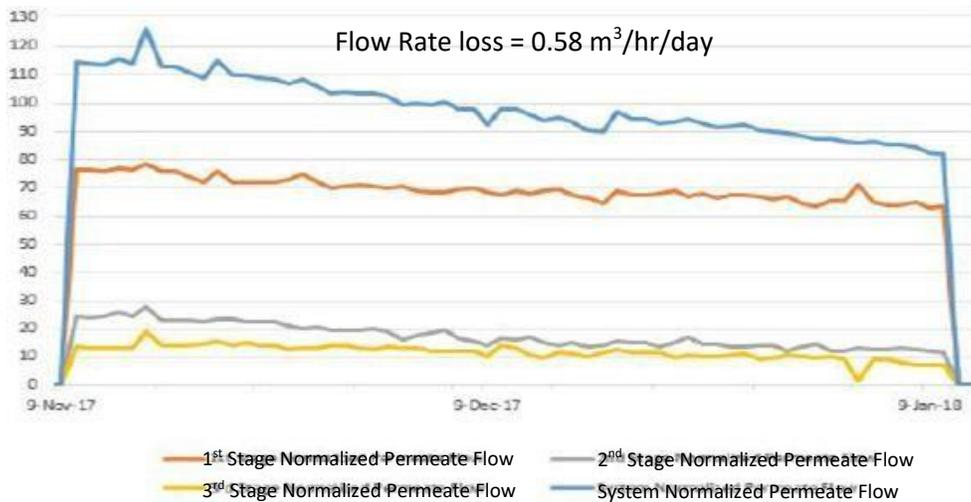
**Figure 6.** Train X Period 2- Normalized Permeate Flow ( $m^3/hr$ )
