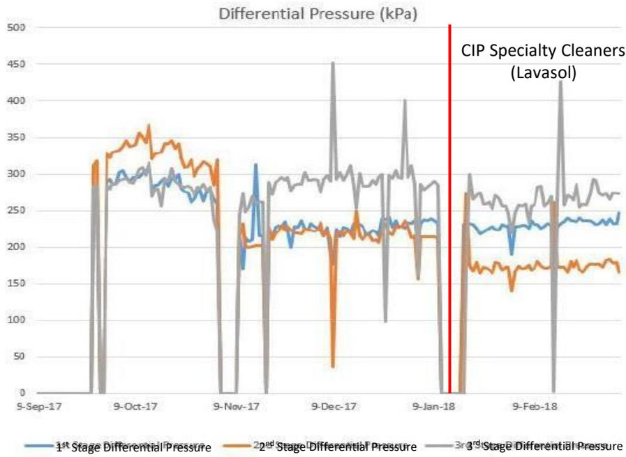
**Figure 8.** Train X: Normalized Differential Pressure variations of the system.
