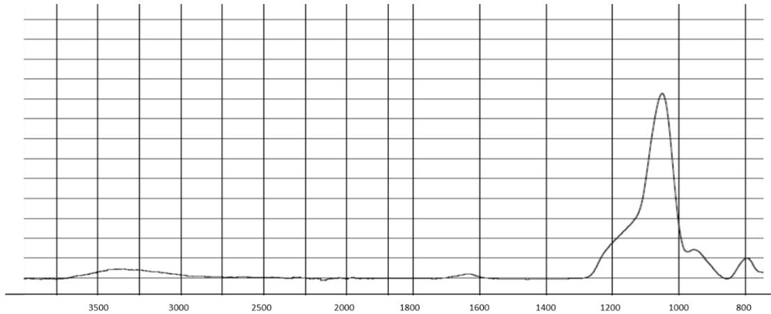
**Figure 3.** FTIR spectrum confirms the presence of Si.
