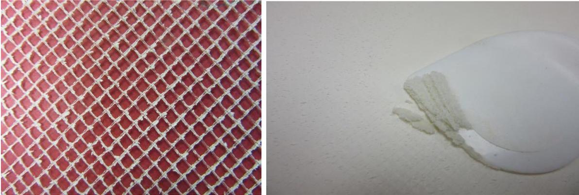
**Figure 1.** White foulant present on feed spacer and membrane surface.
