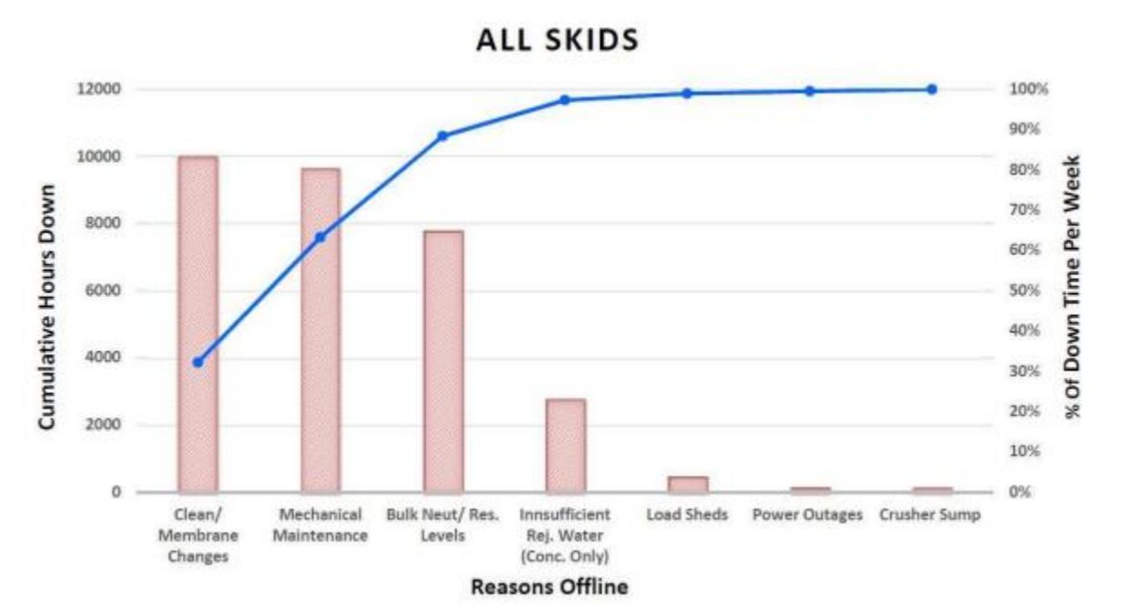
**Figure 10.** Chart to track downtime factors for the RO system at the mining facility.
