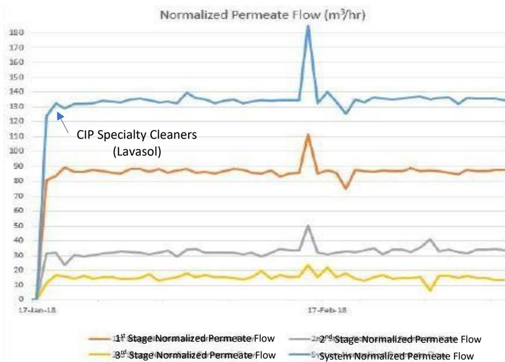
**Figure 7.** Train C Period 3: Normalized Permeate Flow
