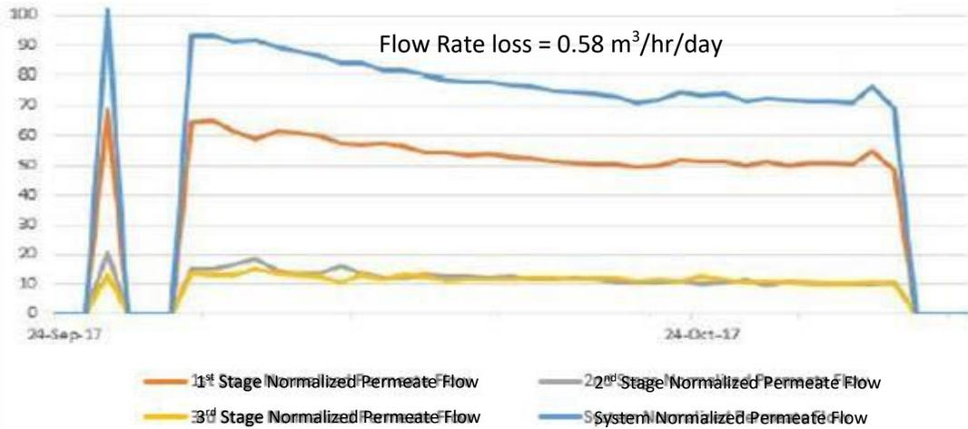
**Figure 5.** Train X Period 1- Normalized Permeate Flow ( $m^3/hr$ )
