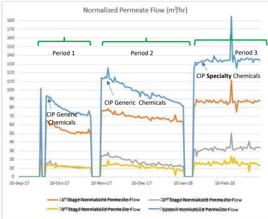
**Figure 4.** Normalized permeate flow split into 3 time periods: Train X.
