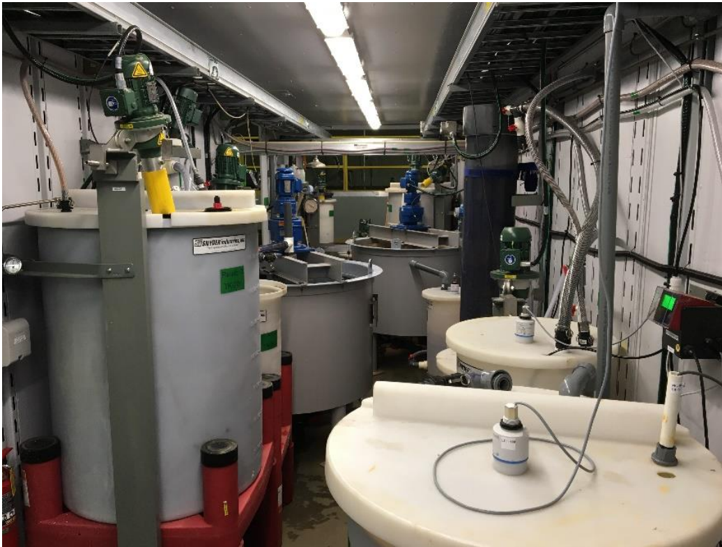
Figure 3: Two-stage HDS pilot plant
