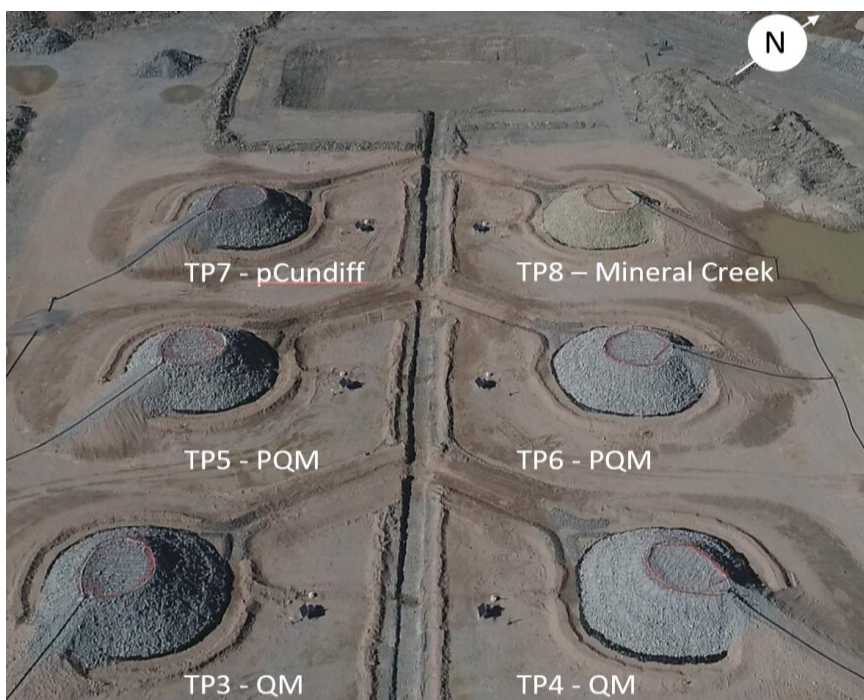
Figure 1. Aerial drone images of the test pads constructed as part of the Bagdad ARD Test Pad Study. Note: QM – Quartz Monzonite; PQM – Porphyry Quartz Monzonite; pCundiff – Precambrian Undifferentiated; Mineral Creek – material from Mineral Creek leach stockpile.
