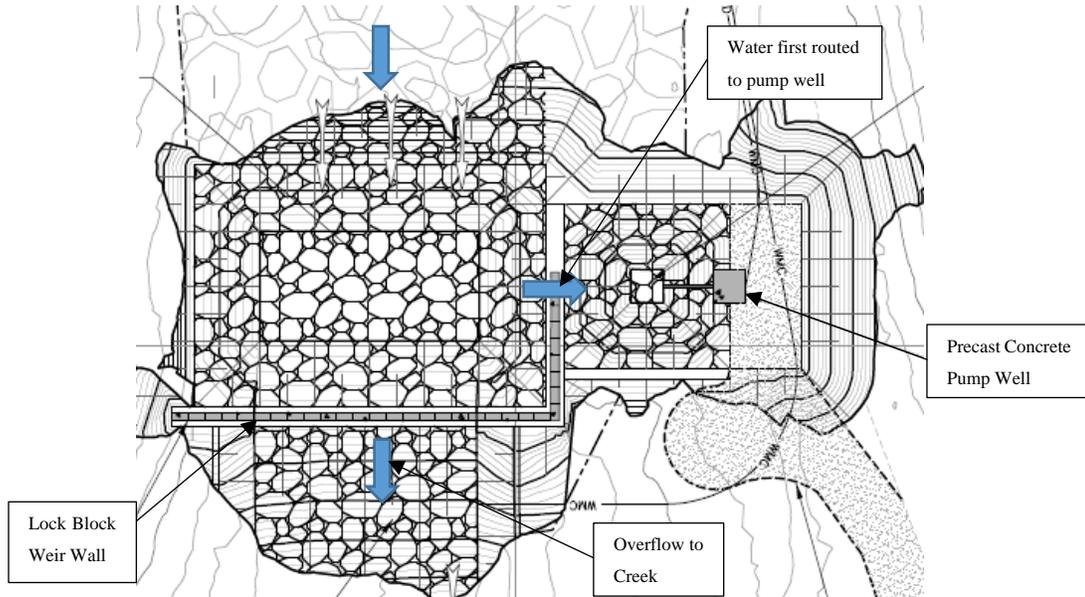
**Figure 7: New dam and intake downstream of pond**
