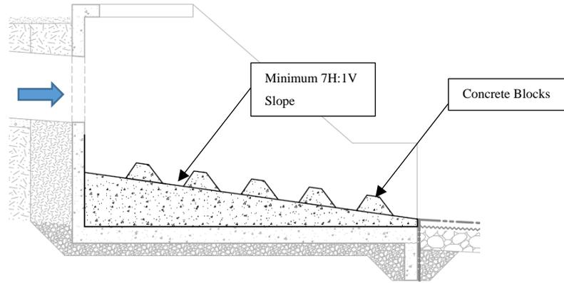
**Figure 9: Chute fish barrier**
