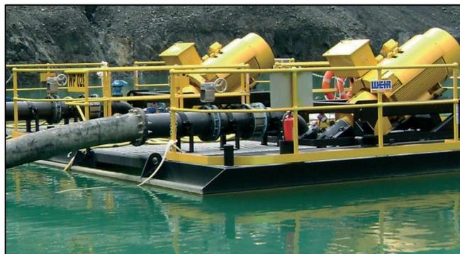
**Figure 6: Floating barge pump**
