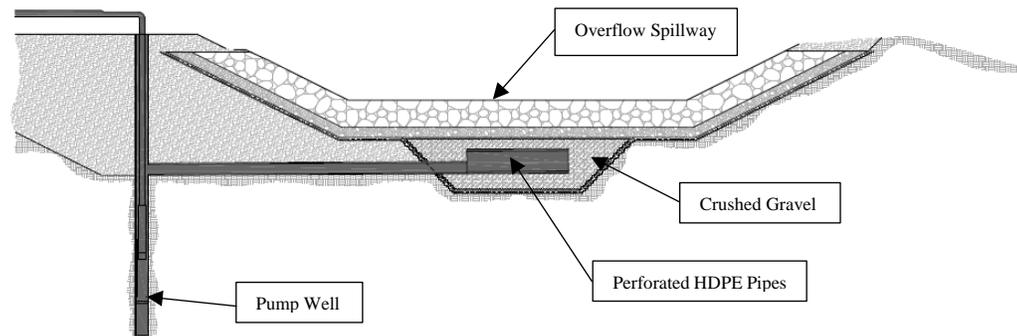
**Figure 3: Infiltration gallery at pond overflow spillway**
